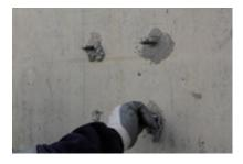
5.- Perform a traction test on the chemical anchors, arriving at 11 KN.
